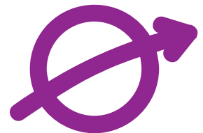
Eau non potable
